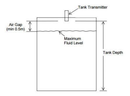
Once you know the Tank Depth and Air Gap, you should convert these units to meters. The default units for the display are in meters, so to simplify the installation of this system you are STRONGLY RECOMMENDED to enter the depths in meters. You can then easily change the units to feet later if you wish.
